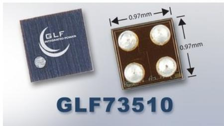
Santa Clara, CA.— January 16, 2018 —[GLF Integrated Power](#), a leading producer of innovative load switch solutions for wearable electronics, introduces the [GLF73510 IQSmart™ IC](#), designed to virtually eliminate wearable and IoT device battery discharge during standby or deep-sleep operation. The GLF73510 consumes an industry-leading ultra-low leakage current ( $I_{SD}$ ) of 2 nA (typ.), as much as 1,000 times less than other manufacturers' chips commonly used in this
