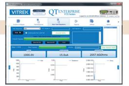
Vitrek's combination cable/harness test solution includes a 950X Series hipot tester, a 964i switch (below) and QT Enterprise software (screen capture).
